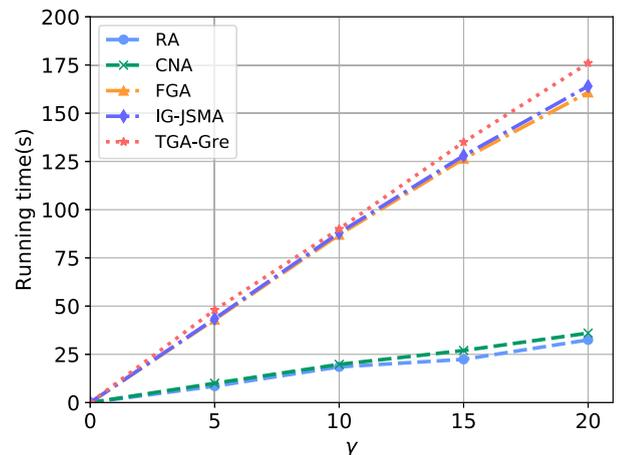
Fig. 6. Runtime of different attack methods performed on the top-100 links with the highest existence probability of DNC.
